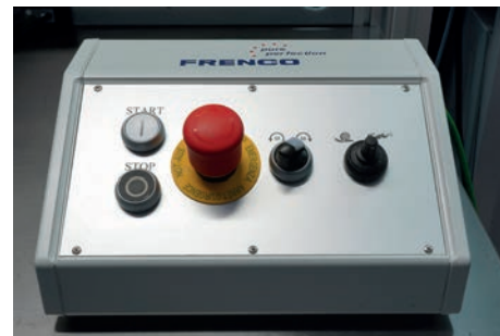
Frenco measuring electronics MEG32 for control and evaluation
