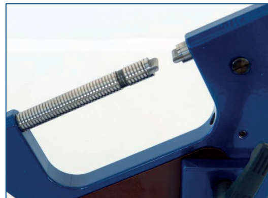
Measuring pin insert (not exchangeable)
