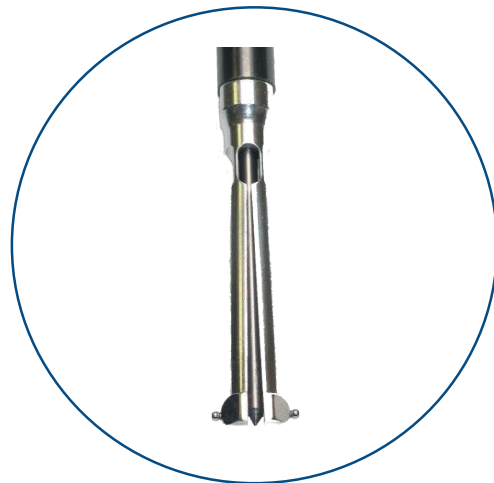
Measuring head with needle and soldered measuring balls
